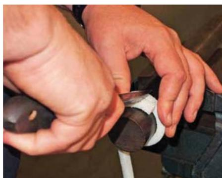
Cutting on a mandrel using "skive cut" 45° angle.
