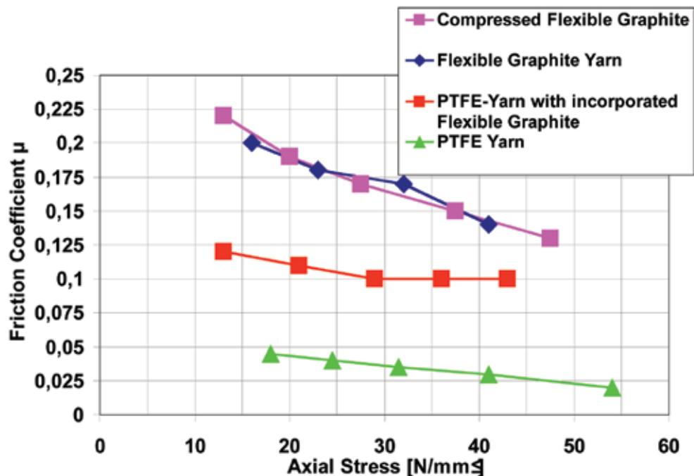
Typical friction coefficients of different packing materials at room temperature
