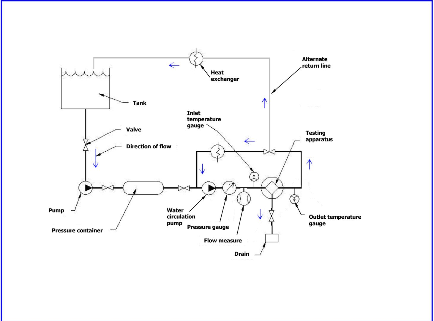
Figure 2 Typical Test Apparatus (Schematic)
