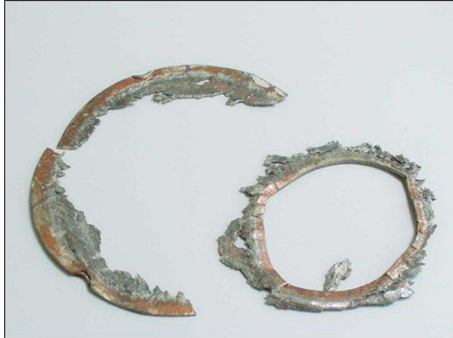
Figure 56: Gasket Chemical Attack
